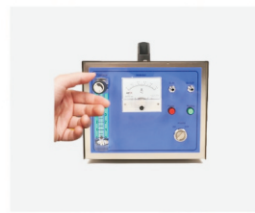
3 Adjust the output air pressure.
